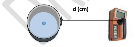
Figure IV-1. Geometry of the measurement. Reproduced courtesy of FORO [IV-4].
